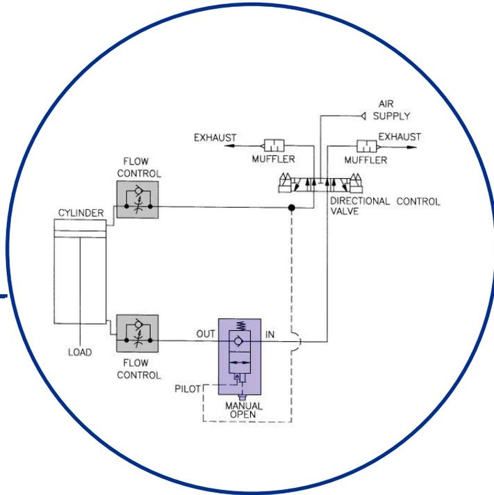
Circuit design to hold cylinder at any stopped position.
