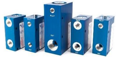
The Nu-Check® valve, designed specifically for pneumatics, is a patented Aladco® product. It was the first check valve on the market with both manual and pilot release capabilities. The unique bubble-tight seal keeps devices in “checked” position. If pressure loss or fluctuation should occur, the valve prevents drifting. To release the seal, depress the manual override button or operate the pilot.
