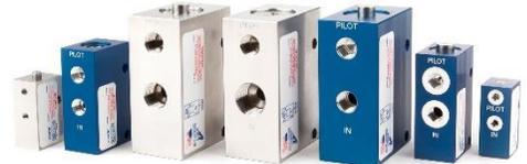
The Equa-Check® valve, designed specifically for pneumatics, is a patented Aladco® product. It is the only check valve on the market with both manual and pilot release capabilities. Equa-Check® valves are pilot operated check valves where the pilot pressure is balanced by the IN chamber pressure. Load balancing systems are a type of application that can benefit from the functions of an Equa-Check® valve.
